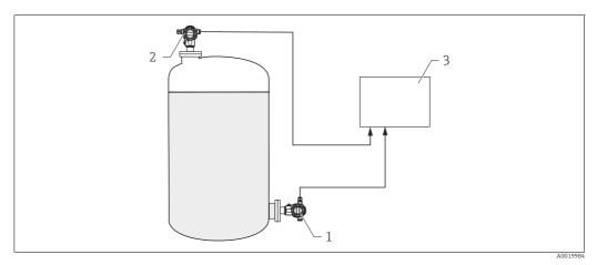
Level measurement in a closed tank with pressure overlay
