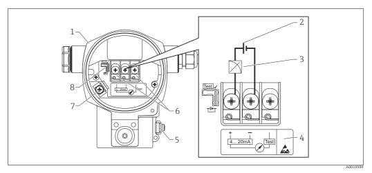
$Terminal\ assignment,\ shown\ here\ with\ aluminum\ housing\ (T14)$
