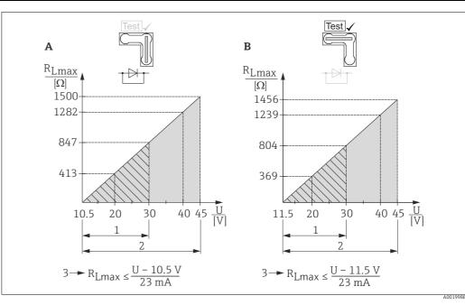
Load diagram, observe the position of the jumper and the explosion protection ( ightarrow extstyle 19, "Measuring a 4 to 20 mA test signal" section.)
