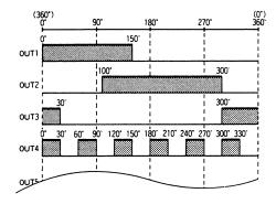
Based on the timing chart, prepare a list that shows the angular data of each program step.
