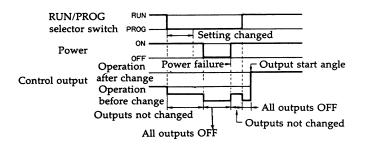
If the output start angle is changed from the previous setting of 0° to 359°, to "no"
