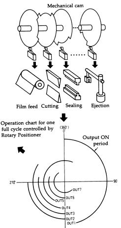
(2) Each control output can be programmed to turn ON/OFF up to 10 times. The Rotary Positioner comes in three types: the H8PR-8 (P) with 8 separate control outputs, the H8PR-16 (P) with 16 separate control outputs, and the H8PR-24 (P), with fully 24 separate control outputs.
