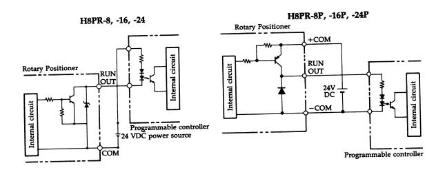
**Note:** Supply the power to the sensor for INHIBIT signal input and output circuit from the same power source.
