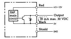
\* This circuit configuration applies to all the outputs.
