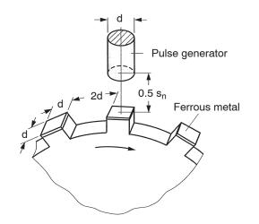
$\begin{array}{rcl} n &=& 1/min \\ n_N &=& Number \mbox{ of trip cams} \\ S_n &=& Rated \mbox{ switching distance} \end{array}$
