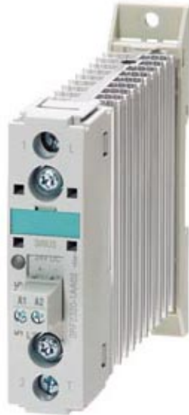
SEMI-COND. CONTACTOR 3RF2,1-PH. AC51 20 A 40 DEGREES C 48-460 V / 24 V DC SCREW TERMINAL
