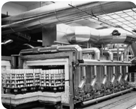
Intermittent shuttle kiln
