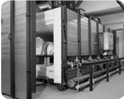
Intermittent shuttle kiln in the ceramics industry
