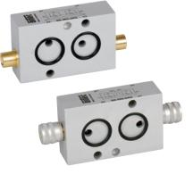
Flow control valves for speed regulation of pneumatically operated actuators. Mounting between NAMUR valve and actuator. Adjustable with screwdriver or manually. The location pin, screws and seals are included.
