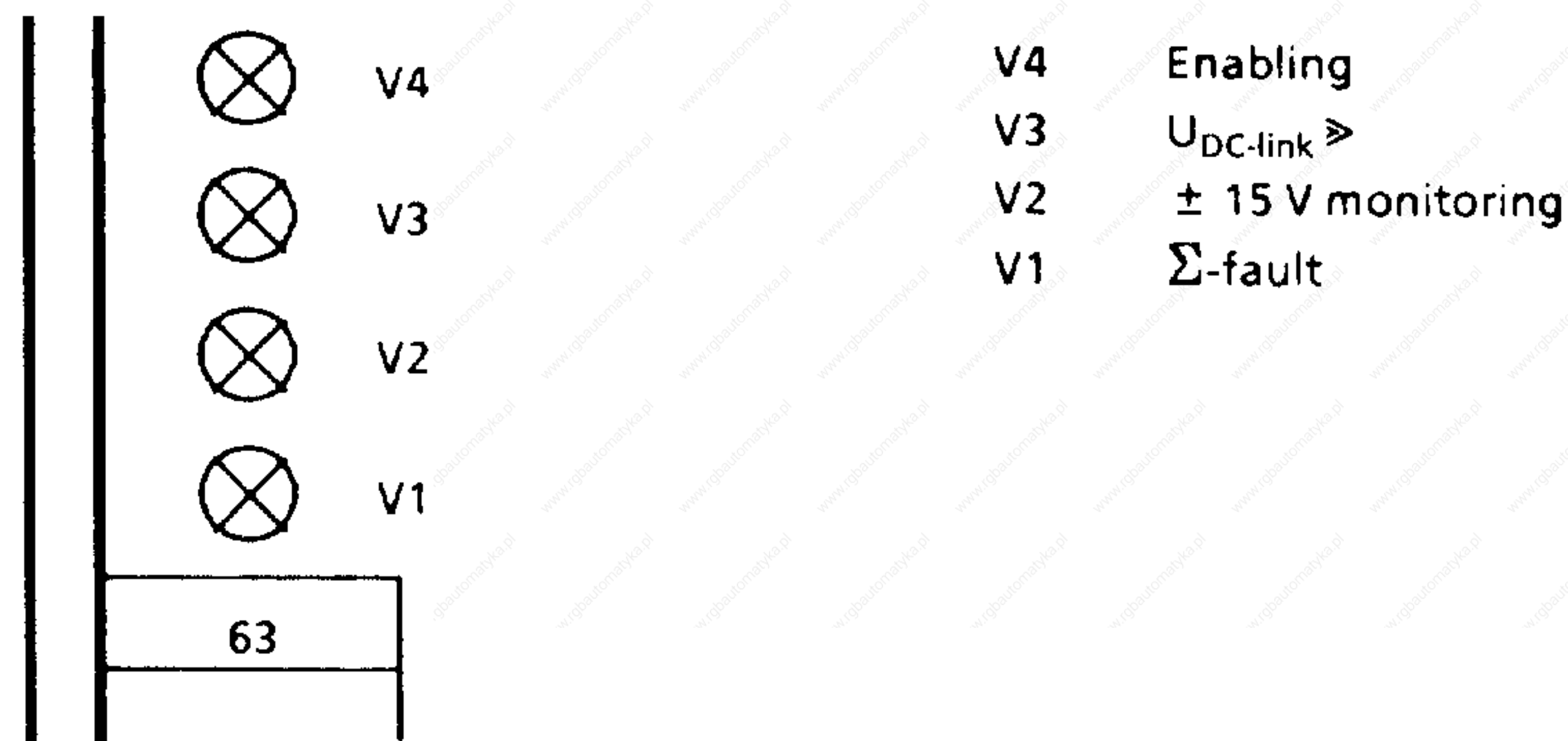
Fig. 3.15 Display elements on power supply module G0
