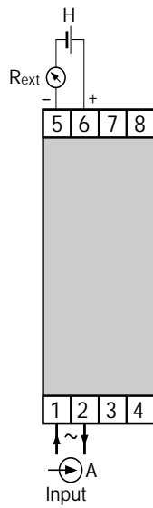
Fig. 7. SINEAX I 503-3.. E as 2-wire converter with 4...20 mA output.
