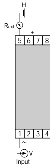
Fig. 8. SINEAX U 504-3.. E as 2-wire converter with 4...20 mA output.
