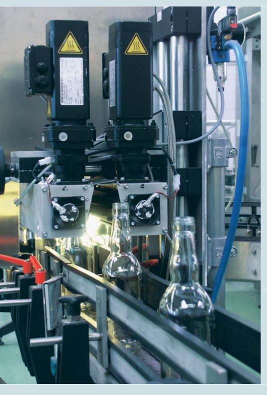
Precision, dynamics and optimum control are characteristic of SEW servomotors. More than 10,000 bottles per hour are turned and checked by planetary gearmotors in phase-synchronous operation and in coordination with MOVIDRIVE® drive inverters.
